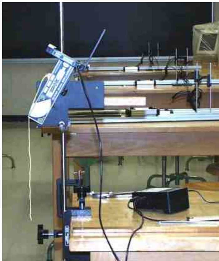
Figure 2: Launcher attached to rod
